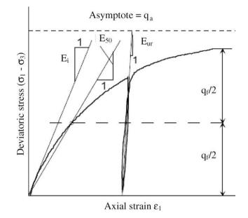
Fig. 6. Hyperbolic stress-strain relationship in primary loading for a standard drained triaxial test (Adapted from Plaxis User's Manual, 2004).
