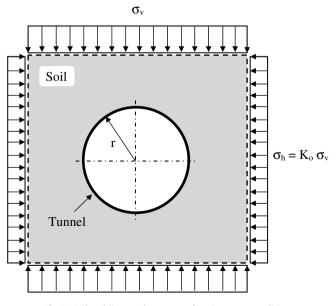
Fig. 2. Soil and liner under a state of in situ stress condition.
