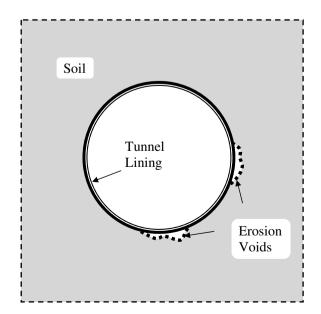
Fig. 1. Existing lining experiencing local support loss as a result of erosion voids.
