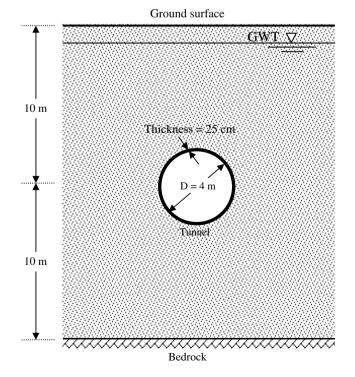
Fig. 3. Problem geometry used in the numerical analysis.
