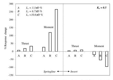
Fig. 16. Percentage change in lining response due to the introduction of voids for F = 16 ( $K_0 = 0.5$ ).
