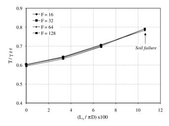
**Fig. 12.** Thrust at the tunnel springline as a function of the void size: ( $K_0 = 0.5$ ).
