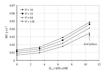
**Fig. 8.** Bending moment at the tunnel springline as a function of the void size:  $(K_o = 0.5)$ .
