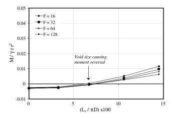
**Fig. 11.** Bending moment at the tunnel invert as a function of the void size:  $(K_0 = 1)$ .
