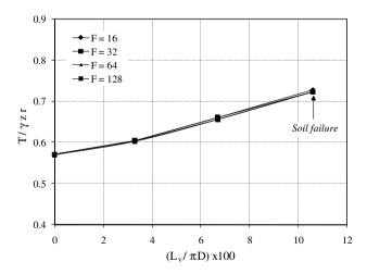
**Fig. 13.** Thrust at the tunnel springline as a function of the void size:  $(K_0 = 1)$ .
