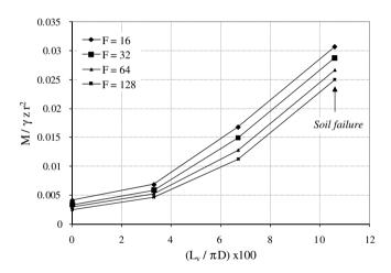
**Fig. 9.** Bending moment at the tunnel springline as a function of the void size:  $(K_o = 1)$ .
