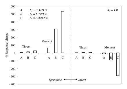
Fig. 17. Percentage change in lining response due to the introduction of voids for F = 16 (K<sub>o</sub> = 1.0).
