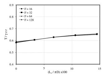
**Fig. 14.** Thrust at the tunnel invert as a function of the void size: ( $K_0 = 0.5$ ).
