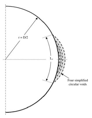
$\ensuremath{\textit{Fig. 5.}}$  Schematic of the simplified geometry of erosion voids located at the springline.
