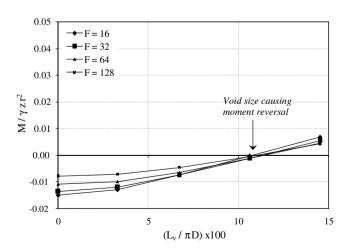
**Fig. 10.** Bending moment at the tunnel invert as a function of the void size: ( $K_o = 0.5$ ).
