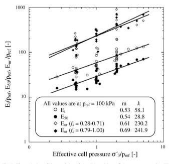
**Fig. 7.** The variation of the modulus of elasticity with confining pressure under CID test condition (Adapted from Kempfert and Gebreselassie, 2006).
