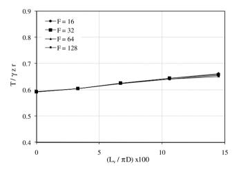
**Fig. 15.** Thrust at the tunnel invert as a function of the void size:  $(K_0 = 1)$ .
