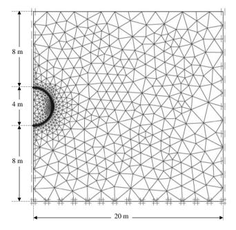
Fig. 4. Finite element mesh used in the numerical analysis. Note: mesh refined around the springline.
